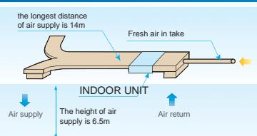
Both fresh air filtration and heating/cooling can be achieved in a single system.
