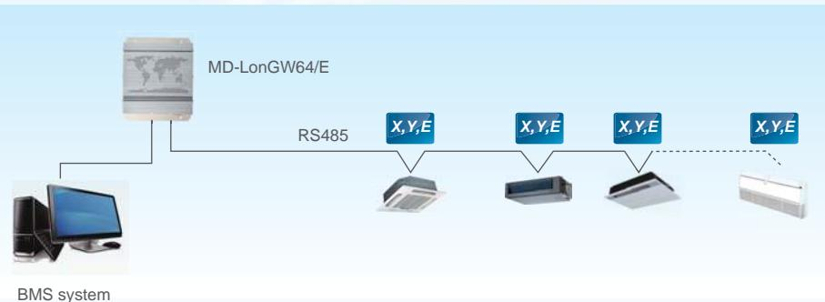
Connection method 2: Only suitable for V4 plus system and connect max.64 indoor units.
