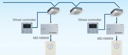
Remote controller or wired controller can control indoor unit.
